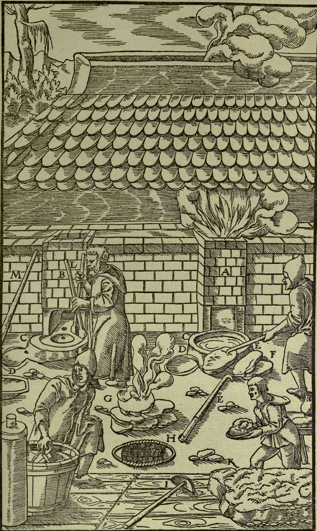
A, B—Two FURNACES. C—FOREHEARTHS. D—DIPPING-POT. THE SMELTER STANDING BY THE FIRST FURNACE DRAWS OFF THE SLAGS WITH A HOOKED BAR. E—HOOKED BAR. F—SLAGS. G—THE ASSISTANT DRAWING A BUCKET OF WATER WHICH HE POURS OVER THE GLOWING SLAGS TO QUENCH THEM. H—BASKET MADE OF TWIGS OF WOOD INTERTWINED. I—RABBLE. K—ORE TO BE SMELTED. THE MASTER STANDS AT THE OTHER FURNACE AND PREPARES THE FOREHEARTH BY RAMMING IT WITH TWO RAMMERS. M—CROWBAR.
