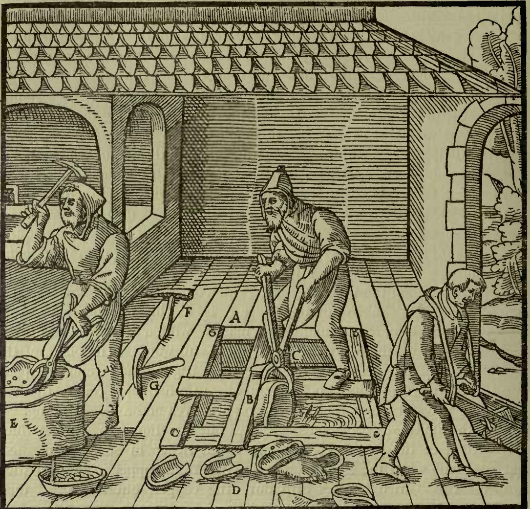
A—TANK. B—BOARD. C—TONGS. D—"DRIED" CAKES TAKEN OUT OF THE TANKS. E—BLOCK. F—ROUNDED HAMMER. G—POINTED HAMMER.
