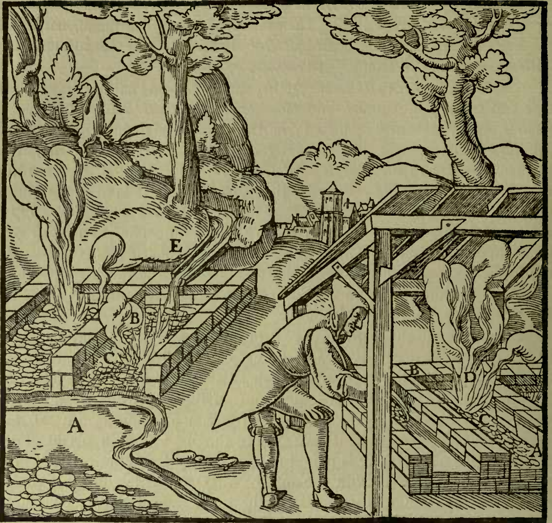
A—AREA. B—WOOD. C—ORE. D—CONE-SHAPED PILES. E—CANAL.
