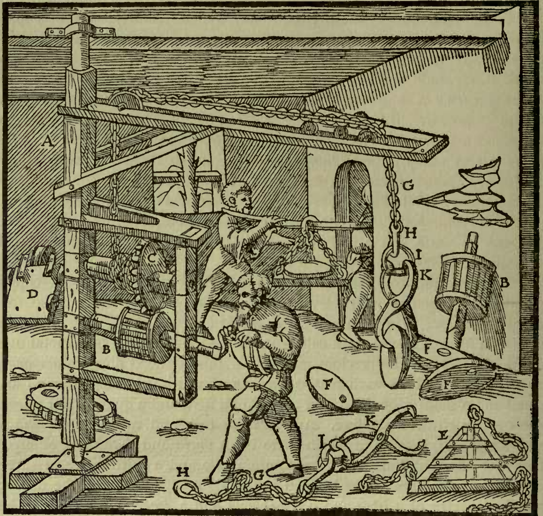
A—CRANE. B—DRUM CONSISTING OF RUNDLES. C—TOOTHED DRUM. D—TROLLEY AND ITS WHEELS. E—TRIANGULAR BOARD. F—CAKES. G—CHAIN OF THE CRANE. H—ITS HOOK. I—RING. K—THE TONGS.
