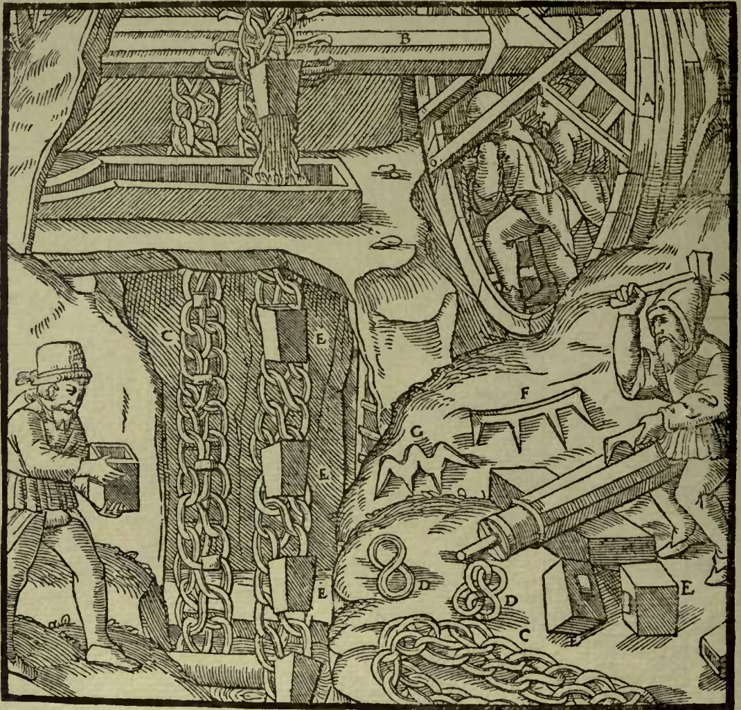
A—WHEEL WHICH IS TURNED BY TREADING. B—AXLE. C—DOUBLE CHAIN. D—LINK OF DOUBLE CHAIN. E—DIPPERS. F—SIMPLE CLAMPS. G—CLAMP WITH TRIPLE CURVES.
