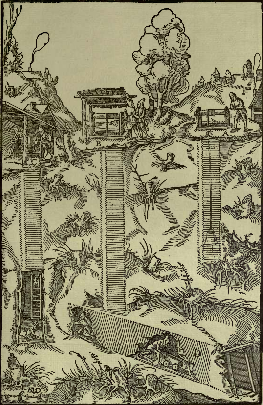
THREE VERTICAL SHAFTS, OF WHICH THE FIRST, A, DOES NOT REACH THE TUNNEL; THE SECOND, B, REACHES THE TUNNEL; TO THE THIRD, C, THE TUNNEL HAS NOT YET BEEN DRIVEN. D—TUNNEL.
