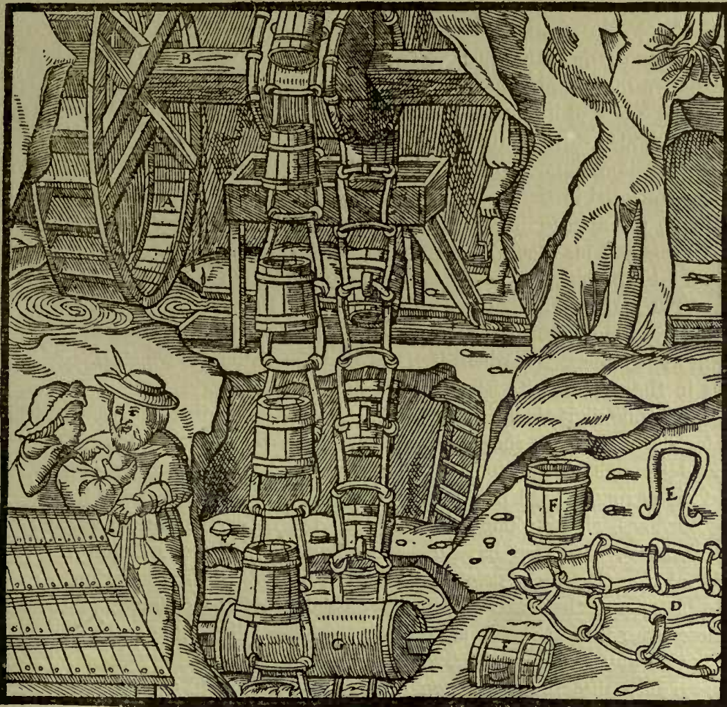
A—WHEEL WHOSE PADDLES ARE TURNED BY THE FORCE OF THE STREAM. B—AXLE. C—DRUM OF AXLE, TO WHICH CLAMPS ARE FIXED. D—CHAIN. E—LINK. F—DIPPERS. G—BALANCE DRUM.
