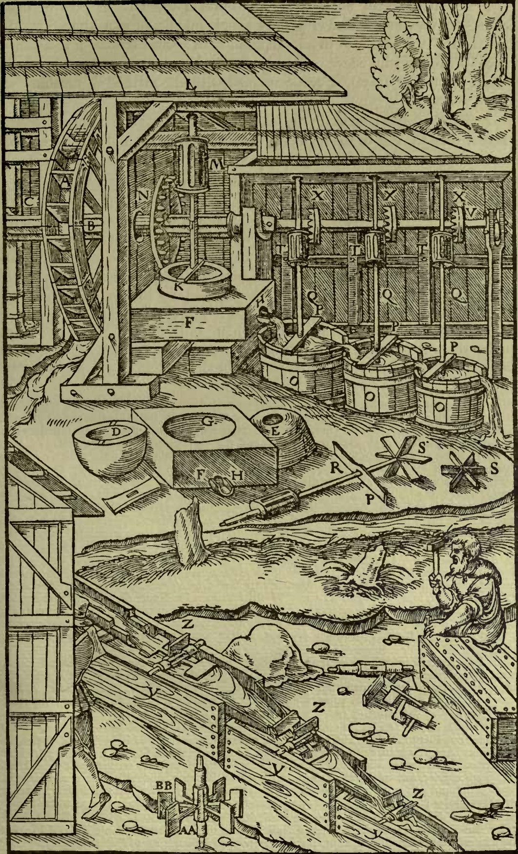
A—WATER-WHEEL. B—AXLE. C—STAMP. D—HOPPER IN THE UPPER MILLSTONE. E—OPENING PASSING THROUGH THE CENTRE. F—LOWER MILLSTONE. G—ITS ROUND DEPRESSION. H—ITS OUTLET. I—IRON AXLE. K—ITS CROSSPIECE. L—BEAM. M—DRUM OF RUNDLES ON THE IRON AXLE. N—TOOTHED DRUM OF MAIN AXLE. O—TUBS. P—THE SMALL PLANKS. Q—SMALL UPRIGHT AXLES. R—ENLARGED PART OF ONE. S—THEIR PADDLES. T—THEIR DRUMS WHICH ARE MADE OF RUNDLES. V—SMALL HORIZONTAL AXLE SET INTO THE END OF THE MAIN AXLE. X—ITS TOOTHED DRUMS. Y—THREE SLUICES. Z—THEIR SMALL AXLES. AA—SPOKES. BB—PADDLES.
