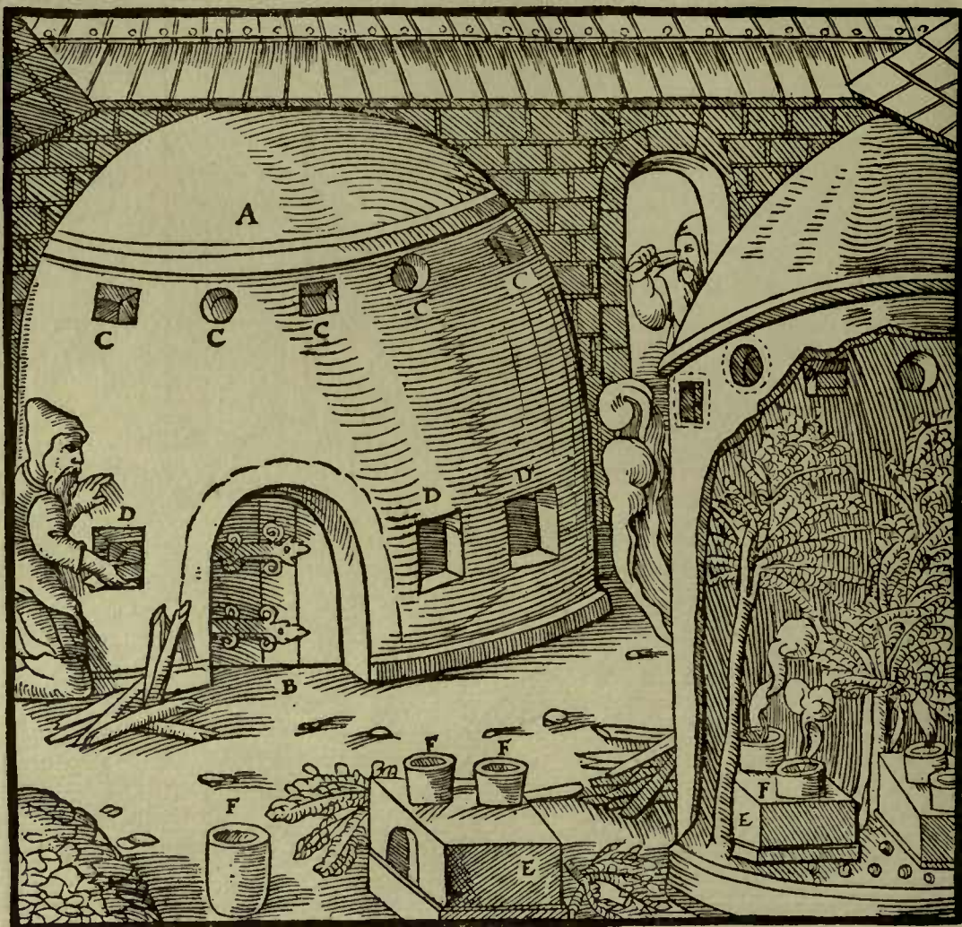
A—ENCLOSED CHAMBER. B—DOOR. C—LITTLE WINDOWS. D—MOUTHS THROUGH THE WALLS. E—FURNACE IN THE ENCLOSED CHAMBER. F—POTS.
