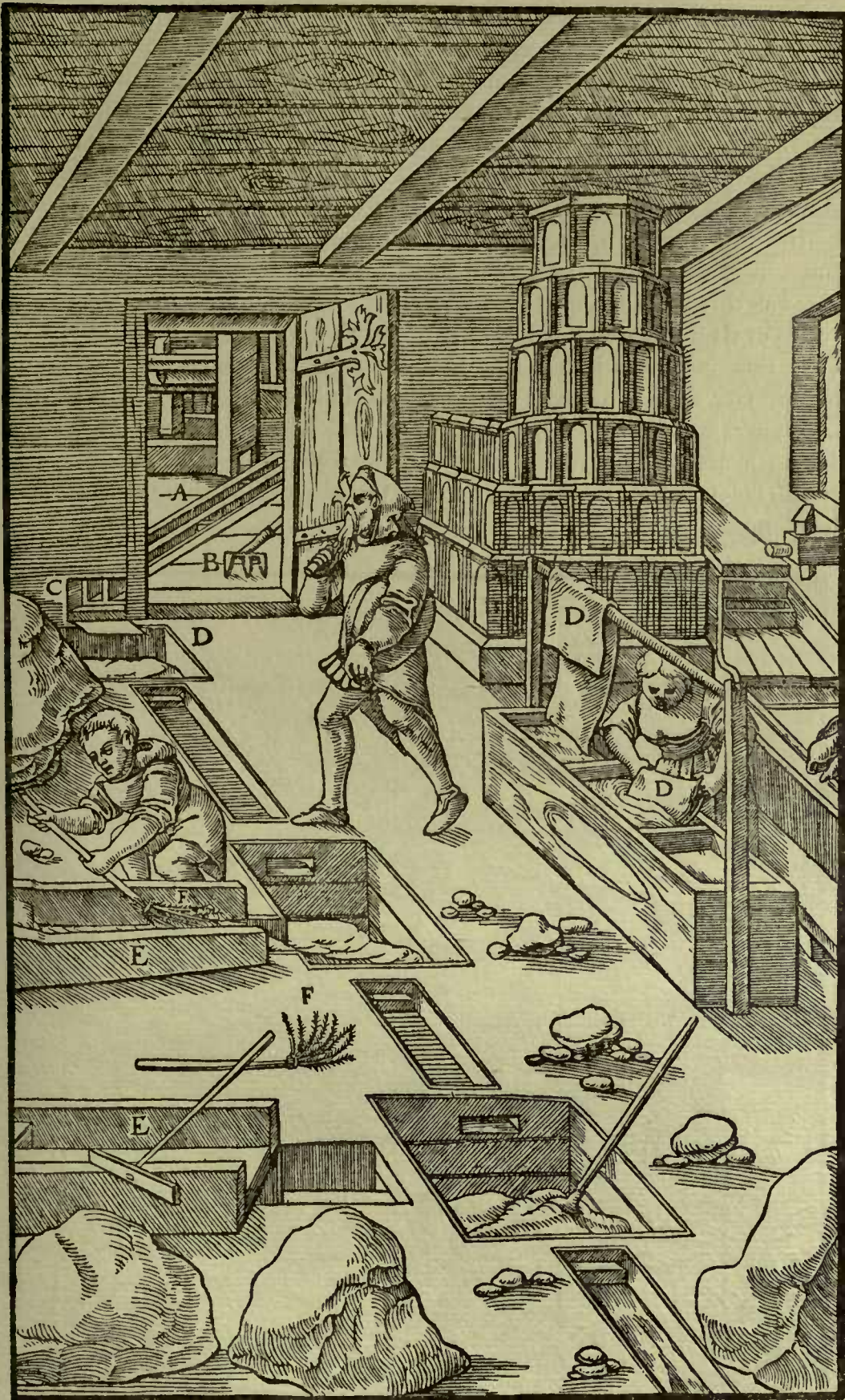
A—LAUNDER FROM THE SCREEN OF THE MORTAR-BOX. B—THREE-TOOTHED RAKE. C—SMALL SETTling-PIT. D—CANVAS. E—STRAKES. F—BROOMS.
