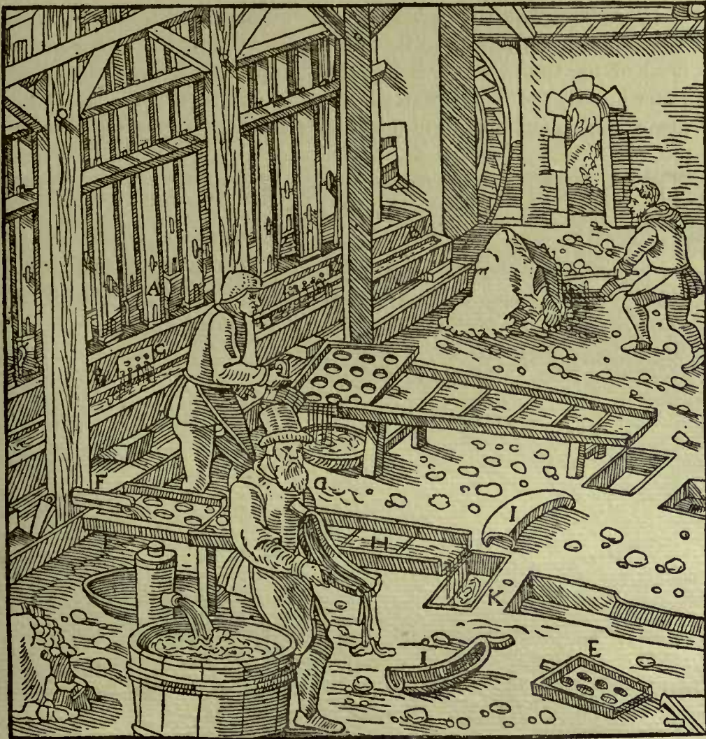
A—STAMPS. B—MORTAR. C—PLATES FULL OF HOLES. D—TRANSVERSE LAUNDER. E—PLANKS FULL OF CUP-LIKE DEPRESSIONS. F—SPOUT. G—BOWL INTO WHICH THE CONCENTRATES FALL. H—CANVAS STRAKE. I—BOWLS SHAPED LIKE A SMALL BOAT. K—SETTLING-PIT UNDER THE CANVAS STRAKE.
