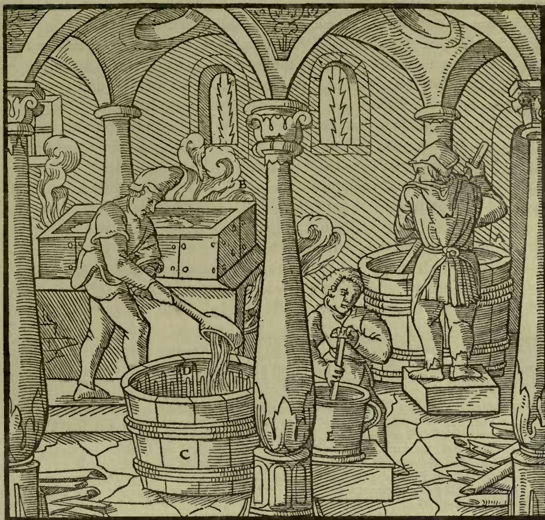
A—VAT IN WHICH THE SODA IS MIXED. B—CALDRON. C—TUB IN WHICH chrysocolla IS CONDENSED. D—COPPER WIRES. E—MORTAR.
