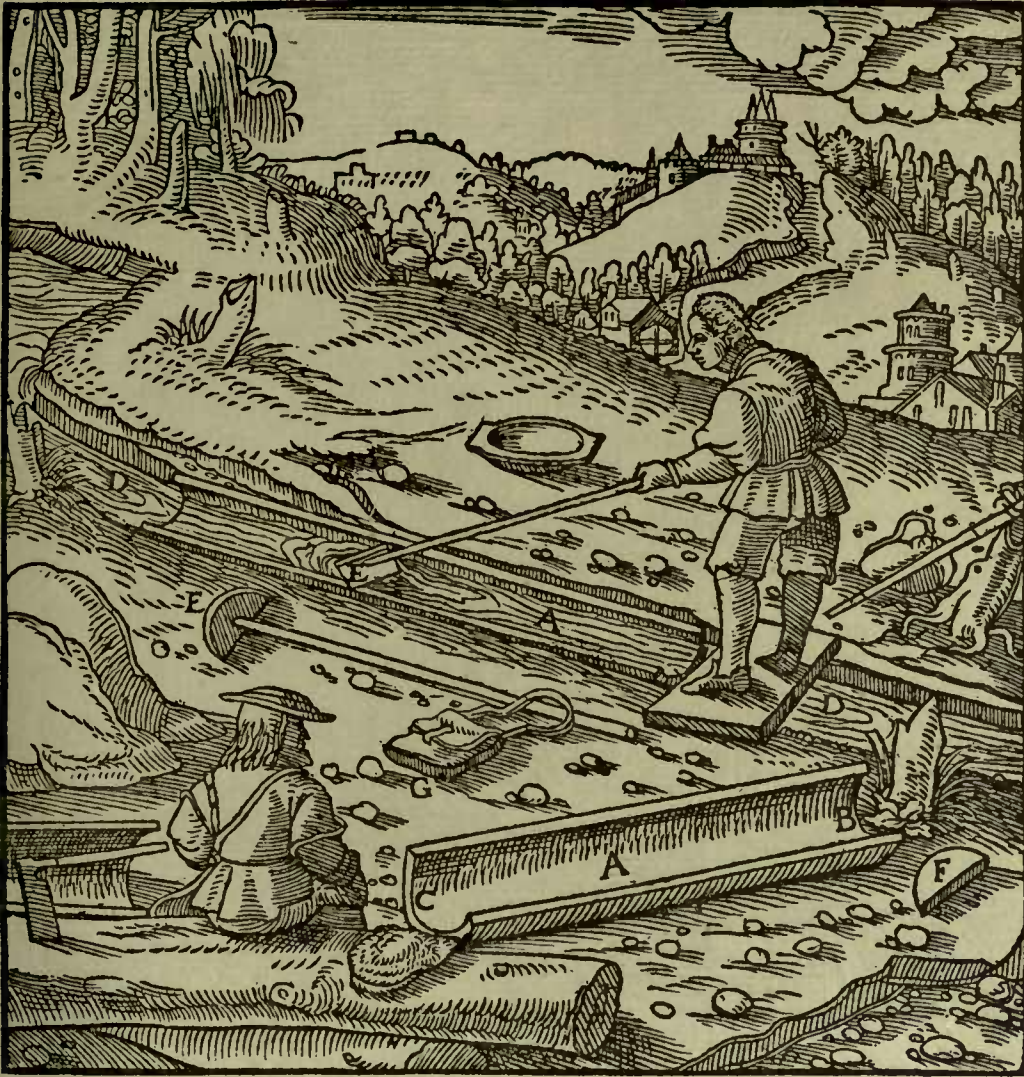
A—TROUGH. B—ITS OPEN END. C—END THAT MAY BE CLOSED. D—STREAM. E—HOE. F—END-BOARD. G—BAG.
