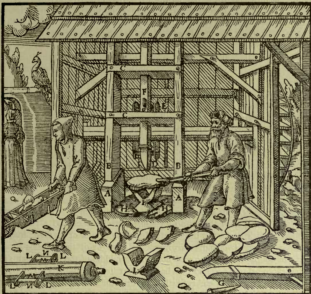
A—BLOCK OF WOOD. B—UPRIGHT POSTS. C—TRANSVERSE BEAMS. D—HEAD OF THE STAMP. E—ITS TOOTH. F—THE HOLE IN THE STAMP-STEM. G—IRON BAR. H—MASSES OF LEAD. I—THE BRONZE SADDLE. K—AXLE. L—ITS ARMS. M—LITTLE IRON AXLE. N—BRONZE PIPE.
