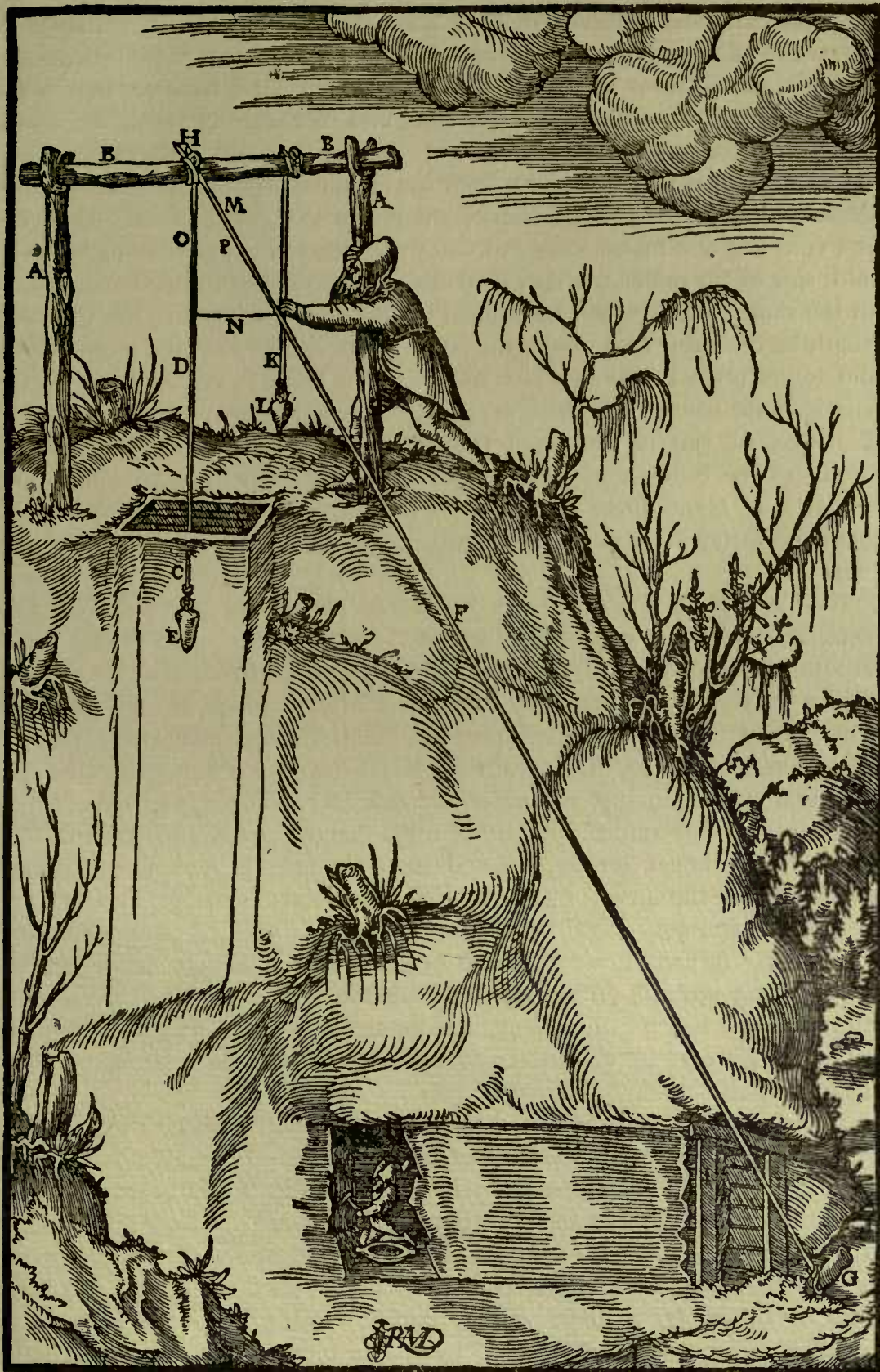
A—UPRIGHT FORKED POSTS. B—POLE OVER THE POSTS. C—SHAFT. D—FIRST CORD. E—WEIGHT OF FIRST CORD. F—SECOND CORD. G—SAME FIXED GROUND. H—HEAD OF FIRST CORD. I—MOUTH OF TUNNEL. K—THIRD CORD. L—WEIGHT OF THIRD CORD. M—FIRST SIDE MINOR TRIANGLE. N—SECOND SIDE MINOR TRIANGLE. O—THIRD SIDE MINOR TRIANGLE. P—THE MINOR TRIANGLE.
