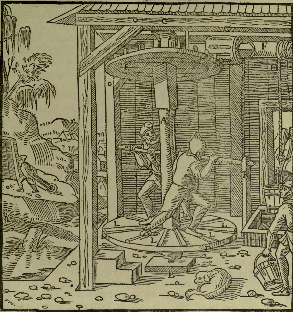
A—UPRIGHT AXLE. B—BLOCK. C—ROOF BEAM. D—WHEEL. E—TOOTHED-DRUM. F—HORIZONTAL AXLE. G—DRUM COMPOSED OF RUNDLES. H—DRAWING ROPE. I—POLE. K—UPRIGHT POSTS. L—CLEATS ON THE WHEEL.
