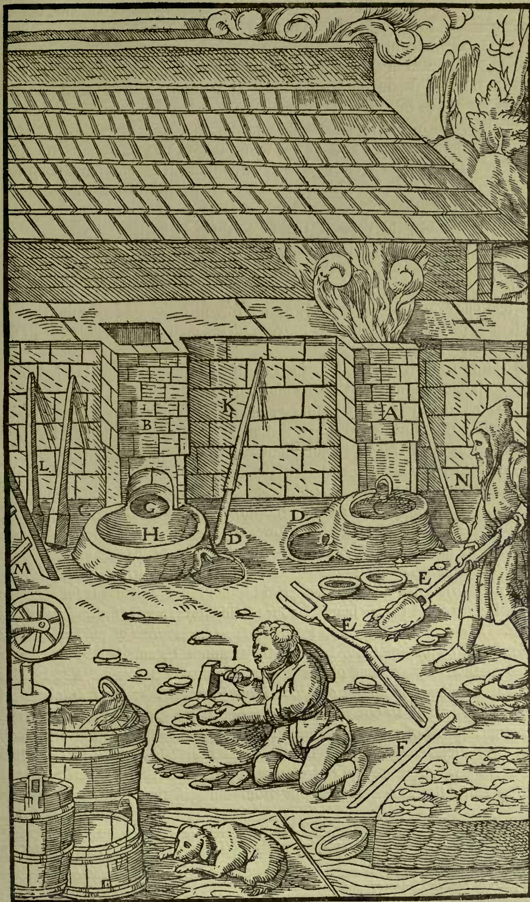
A, B—Two furnaces. C—FOREHEARTH. D—DIPPING-POTS. THE MASTER STANDS AT THE ONE FURNACE AND DRAWS AWAY THE SLUGS WITH AN IRON FORK. E—IRON FORK. F—WOODEN HOE WITH WHICH THE CAKES OF MELTED PYRITES ARE DRAWN OUT. G—THE FOREHEARTH CRUCIBLE: ONE-HALF INSIDE IS TO BE SEEN OPEN IN THE OTHER FURNACE. H—THE HALF OUTSIDE THE FURNACE. I—THE ASSISTANT PREPARES THE FOREHEARTH, WHICH IS SEPARATED FROM THE FURNACE THAT IT MAY BE SEEN. K—BAR. L—WOODEN RAMMER. M—LADDER. N—LADLE.
