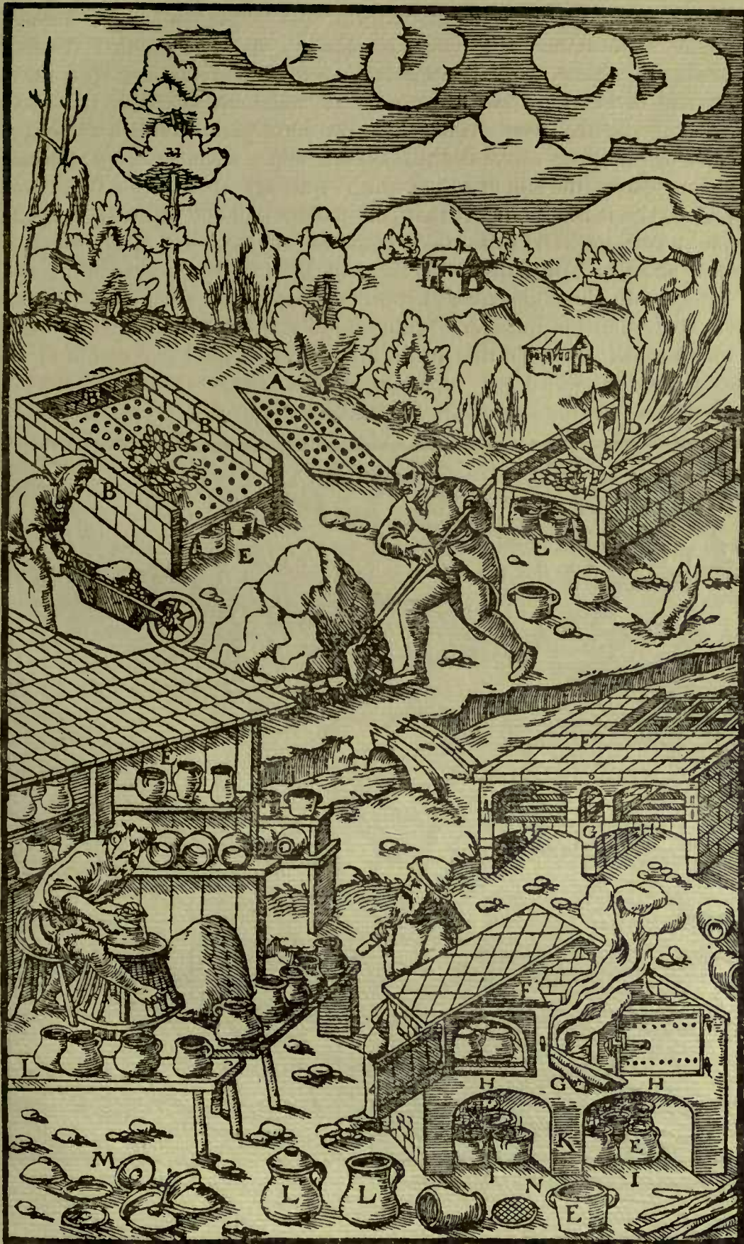
A—IRON PLATES FULL OF HOLES. B—WALLS. C—PLATE ON WHICH ORE IS PLACED. D—BURNING CHARCOAL PLACED ON THE ORE. E—POTS. F—FURNACE. G—MIDDLE PART OF UPPER CHAMBER. H—THE OTHER TWO COMPARTMENTS. I—DIVISIONS OF THE LOWER CHAMBER. K—MIDDLE WALL. L—POTS WHICH ARE FILLED WITH ORE. M—LIDS OF SAME POTS. N—GRATING.
