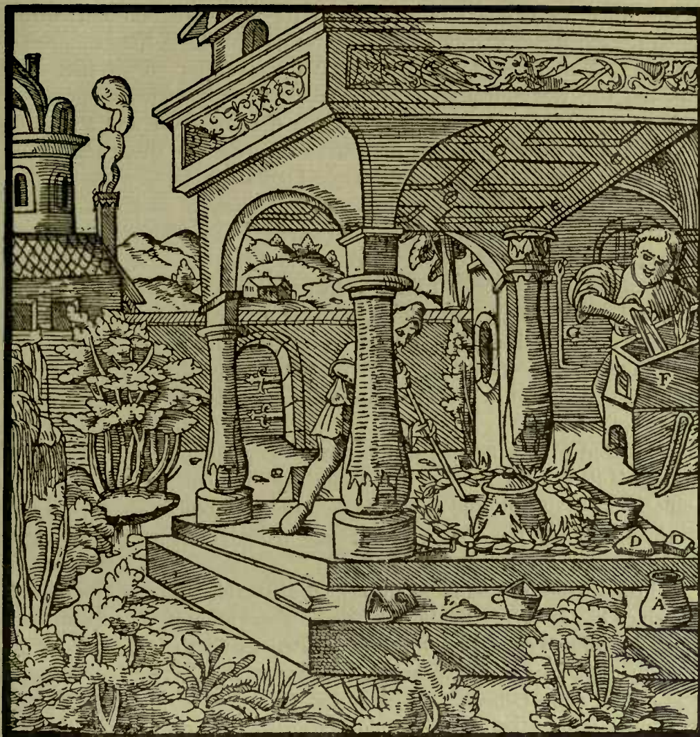
A—Pot. B—CIRCULAR FIRE. C—CRUCIBLES. D—THEIR LIDS. E—LID OF THE POT. F—FURNACE. G—IRON ROD.
