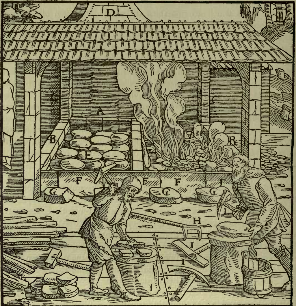
A—BACK WALL. B—WALLS AT THE SIDES. C—UPRIGHT POSTS. D—CHIMNEY. E—THE CAKES ARRANGED. F—IRON PLATES. G—ROCKS. H—RABBLE WITH TWO PRONGS. I—HAMMERS.
