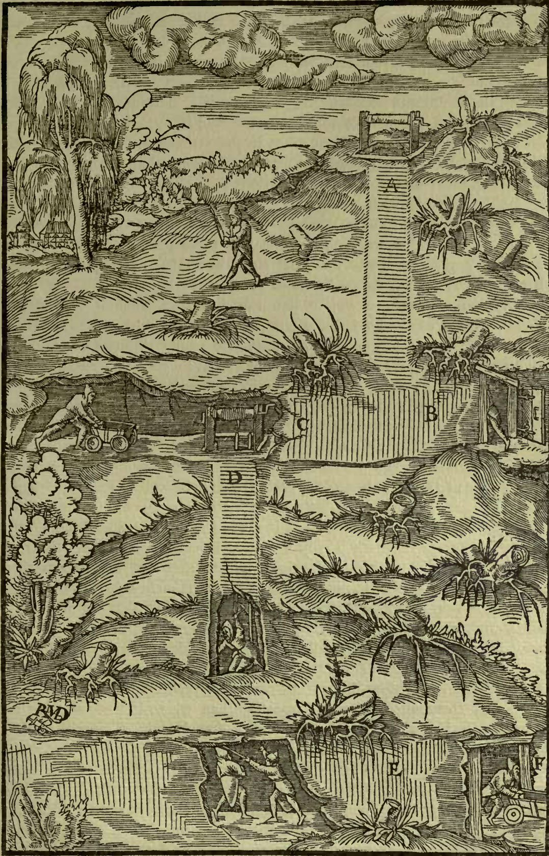
A—SHAFT. B, C—DRIFT. D—ANOTHER SHAFT. E—TUNNEL. F—MOUTH OF TUNNEL.
