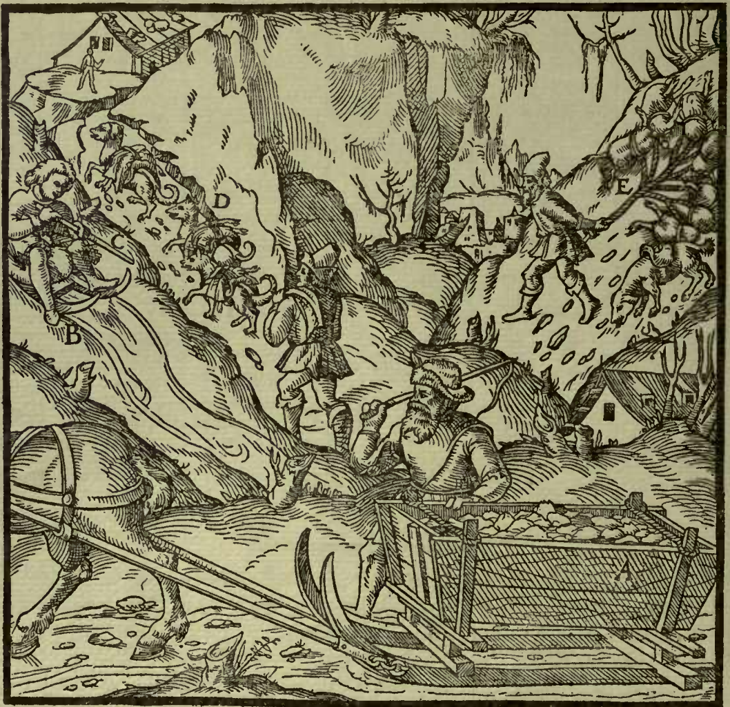
A—SLEDGE WITH BOX PLACED ON IT. B—SLEDGE WITH SACKS PLACED ON IT. C—STICK. D—DOGS WITH PACK-SADDLES. E—PIG-SKIN SACKS TIED TO A ROPE.
