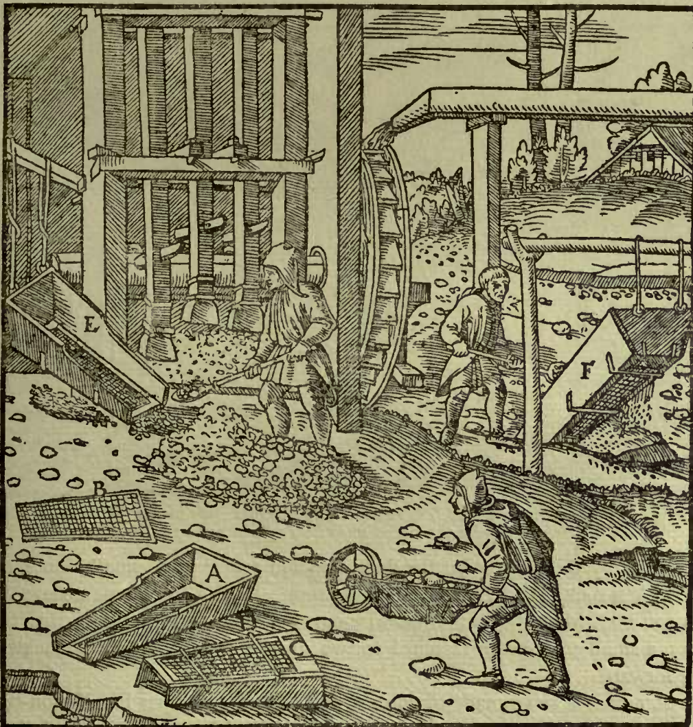
A—BOX LAID FLAT ON THE GROUND. B—ITS BOTTOM WHICH IS MADE OF IRON WIRE. C—BOX INVERTED. D—IRON RODS. E—BOX SUSPENDED FROM A BEAM, THE INSIDE BEING VISIBLE. F—BOX SUSPENDED FROM A BEAM, THE OUTSIDE BEING VISIBLE.
