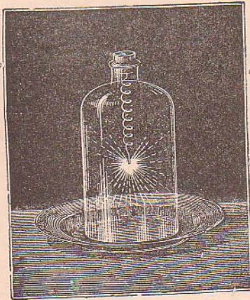
BURNING STEEL AND SULPHUR OR PHOSPHORUS IN OXYGEN.
