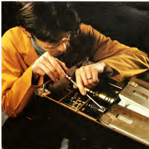
Connection of the two bellows to the driving lever
