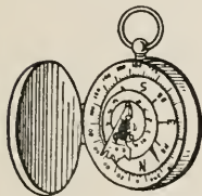
Fig. 33. A Watch-Case Sun-Dial and Compass
