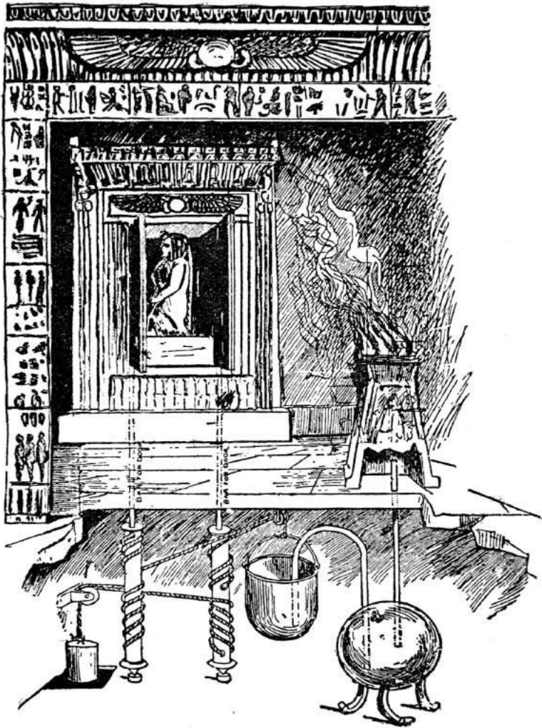
APPARATUS FOR OPENING THE DOORS OF A SHRINE WHEN A FIRE IS LIGHTED ON AN ALTAR
