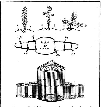
I regret that I have not drawn the plan of the cage quite accurate, for the three small cage parts should be shown broader, to allow each part to swing into each other. The arrows point to where the spring hinges are fitted.
