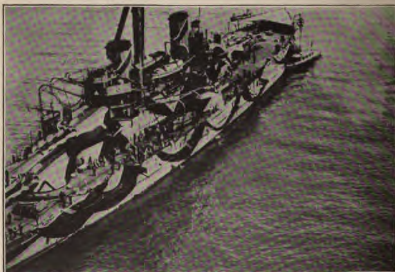
Figs. 93 and 94. — Attempts at distortion of outline which preceded the adoption of geometrical-optical illusions for ships.
