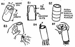
The tape was placed in position (see cross-sectional Fig 81), and the tube was then wound tightly with ordinary flesh-coloured surgical adhesive plaster, so as to fix the tape in position and also provide a flesh-coloured exterior (Fig. 82). The finished product was thoroughly rubbed with French chalk and the surplus brushed off, this to prevent stickiness from the plaster. Finally, the tape was coloured in each fake to match the silk with which it would be loaded for the trick.
