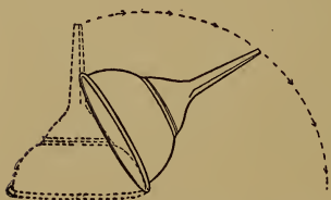
FIG. 1. HOW TO COVER A FUNNEL, CORNUCOPIA, ETC., WITH A FILM
