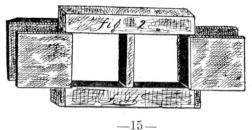
other; see Figs. 1 and 3. The two side base blocks, J J, are nailed to each end of the box, and appear to the uninitiated as a simple decoration. The left back and two front doors are now hinged on so they will open outwardly as illustrated in Fig. 2, and a thumb tack is affixed to each to facilitate their being opened and closed.
