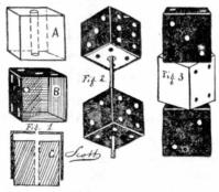
Holes are bored through the centers of each die as illustrated at A of Fig. 1. B, of Fig. 1 pictures the shell and its interior. A hole is bored through the center of the side which is opposite the open end.
