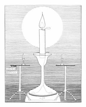
The Ever Ready Co. have placed on the market an electric gas-lighter made like a flash-lamp at 5/6. The parts of one of these may be used to construct the device. The battery provided will then light the candle 7,000 times!
