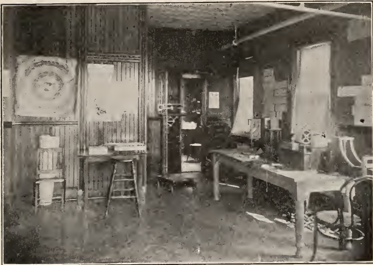
FIG. 1. A CORNER OF THE PSYCHOLOGICAL LABORATORY WHERE DR. GODDARD CONDUCTS HIS EXPERIMENTS. There are shown an ergograph, a chronoscope, which measures intervals of time to one thousandth of a second, a dark room for photographic work, an automotograph for recording involuntary movements of hand and arm, a target for testing precision in motor control, etc.
