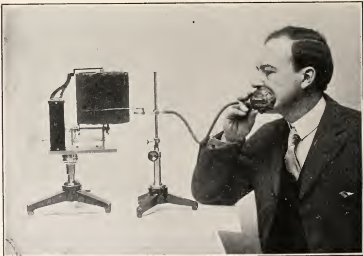
FIG. 1. RECORDING THE VOICE. The waves from the mouth proceed down the wide tube to the rubber membrane at the end. The vibrations of the membrane are recorded by a straw lever on a surface of smoked paper around a revolving cylinder.
