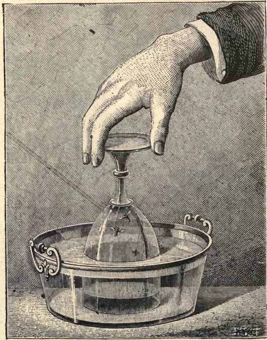
Fig. 52.—The principle of the diving-bell.
