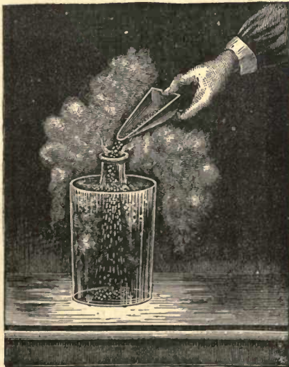
Fig. 395.—Experiment showing affinity between arsenic and chlorine.
