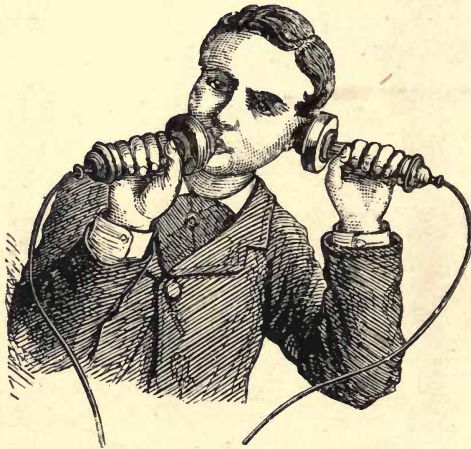
Fig. 194.—Mode of using the Telephone.
