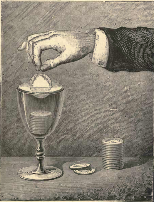
Fig 65.—Experiment on the convexity of a meniscus.
