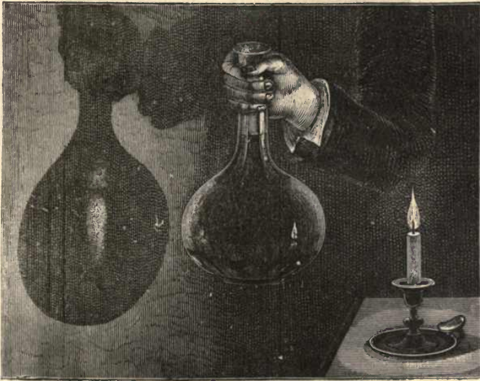
Fig. 90.—A water-bottle employed as a convergent lens.
