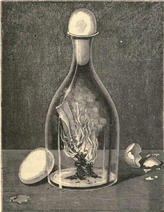
Fig. 43.—Hard boiled egg, divested of its shell, passing through the neck of a glass bottle, under the influence of atmospheric pressure.
