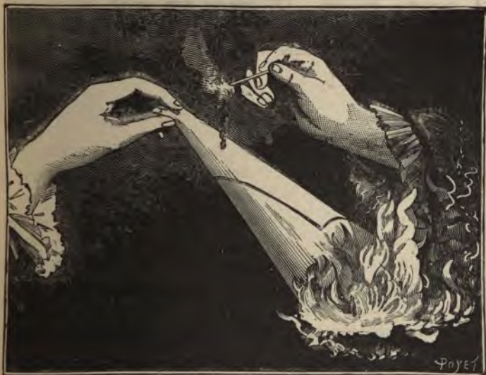
Fig 83.—Production of Gas with a Paper Cone.
