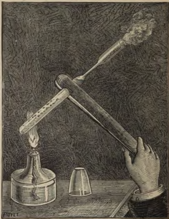
Fig. 81.—Preparation of a Saturated Solution of Sulphate of Soda.
