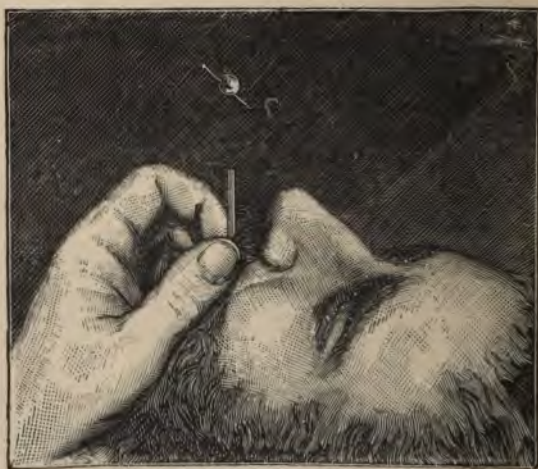
Fig. 36.—Pea sustained in the Air by blowing through a Tube.
