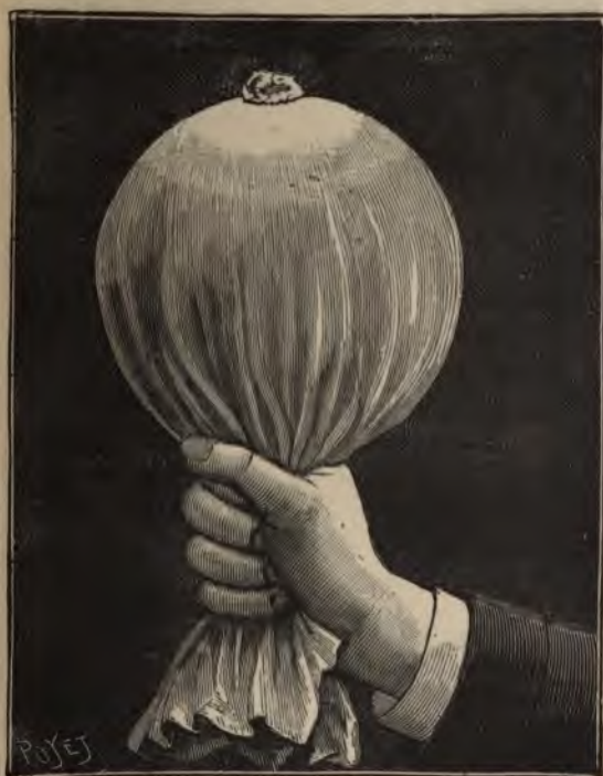
Fig. 56.—A Burning Coal placed on a Handkerchief wrapped round a Copper Globe. The Handkerchief is not scorched.
