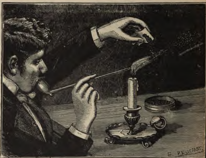
Fig. 78.—Iron Filings burning in a Jet of Air.
