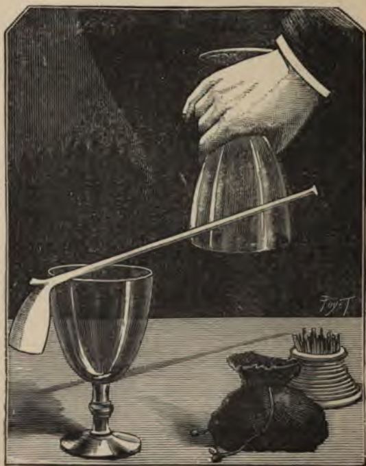
Fig. 74.—Pipe attracted by an Electrified Glass.
