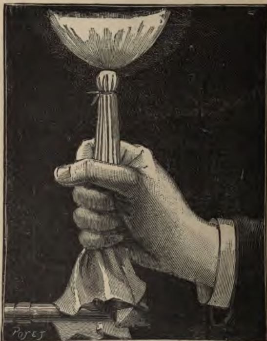
Fig. 57.—Gas Jet (Metal) wrapped in a Cambric Handkerchief, tightly stretched. The Flame will burn above the Handkerchief without injuring it.
