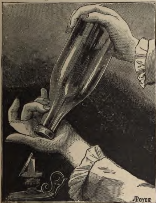
Fig. 51.—Mode of holding the Bottle in order to extinguish, or blow aside, the Flame.
