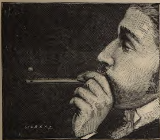
Fig. 37.—Bread Pellet sustained by a Current of Air.
