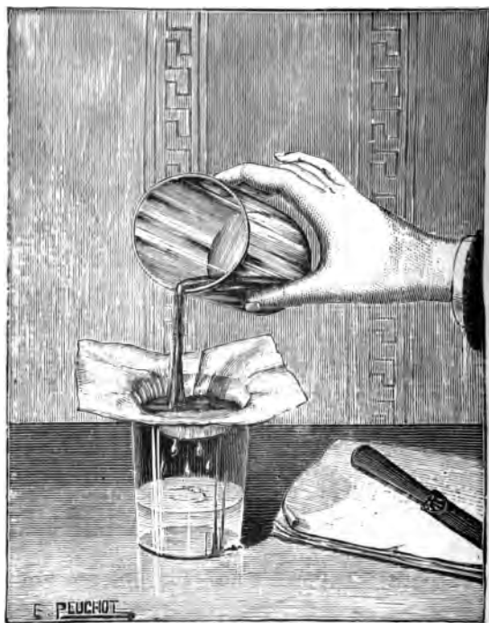
Fig. 5.--The Blotting-paper Filter.
