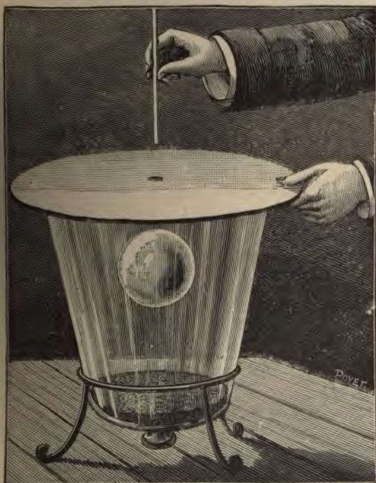
Fig. 79.—Soap-bubble floating on the Surface of a Layer of Carbonic Acid Gas.
