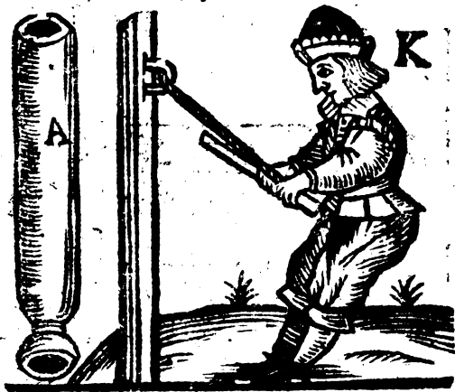
5. The manner of driving a Rocket, with the Instruments belonging thereto.
