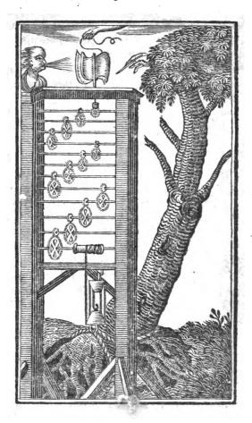
The whole force of this engine doth consist in two double pullics, twelve wheels, and a sail. One of these pullies at the bottom will diminish half of the weight, so that it shall be but as 2000000000, and the other pulley will
