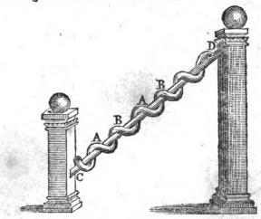
Where you see there is a cylinder A A, and a spiral cavity or pipe twining about it, according to equal revolutions
