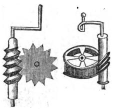
For the composure of which, instead of the female, or concave screw, there must be a little wheel with some notches in it, equivalent to teeth\*, by which the other may take hold of it, and turn it round, as in these other figures.
