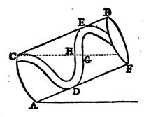
Where A B represents a screw covered over, C D E one helix, or revolution of it, C D the ascending side, E D the descending side, the point D the middle. The horizontal line C F, shewing how much of the helix is filled with water, viz. of the ascending side, from C the beginning of the helix, to D the middle of it; and on the descending side,
