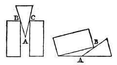
Therefore Ubaldus hath more exactly applied the several parts of it according to this form, that the point A, should be as the common fulciment, in which both the sides do meet, and (as it were) uphold one another; the points B, and C, representing that part of the leavers where the weight is placed.
