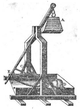
That great box or cavity at A, is supposed to be full of some heavy weight, and is forced up by the turning of the axis and spokes B C. The stone or bullet to be discharged, being in a kind of sling at D; which when the greater weight A descends, will be violently whirled upwards, till that end of the sling at E, coming to the top will fly off, and discharge the stone as the skilful artist should direct it.
