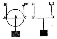
Let AC represent the diameter of a lower pulley, on whose centre at B the weight is fastened, one end of the cord being tied to a hook at D. Now it is evident, that half the weight is sustained at D, so that there is but the other half left to be sustained by the power at E: it being all one, as if the weight were tied unto the middle of the balance FG, whose ends were upheld by two several strings, FH, and GI.
