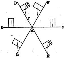
Where A is supposed to be the place of the prop, or fulciment; BC, a leaver which stands horizontally; the power and the weight belonging unto it being equal, both in themselves, and also in their distances from the prop.
