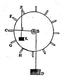
Suppose AB for the semidiameter of the axis or cylinder, and AC for the semidiameter of the rundle with
