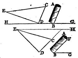
then the inclination of the revolutions in it will be increased by the angle EDH; though these revolutions will still remain in a kind of ascent, so that water cannot be turned through them.
