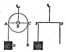
The diameter AC being as the beam of a balance, of which B is the prop or centre; now the parts A and C being equally distant from this centre, therefore the power at E must be equal to the weight at D; it being all one, as if the power and the weight were fastened by two several strings, at the ends of the balance FG.
