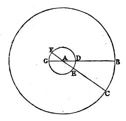
Let the line GAB represent a balance, or leaver; the weight being supposed at the point G, the fulciment at A, and the power sustaining the weight at B. Suppose the point G, unto which the weight is fastened, to be elevated unto F, and the opposite point B to be depressed unto C;
