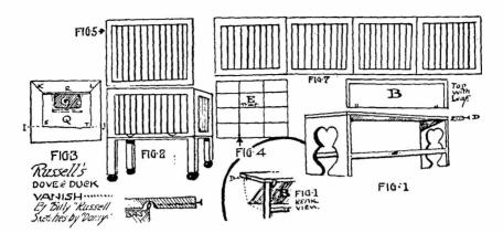
table rail C. E is a trap in the table top (4). This table top is divided into squares by tacking on metallic ribbons or metal strips as the lines show. In one of these squares the trap is placed. E. is a window bolt release. When pulled, trap E raises (spring hinges) into cage leaving trap open for performer to insert birds. 3 shows the under side of the table top (4). Q is a black canvas bag to hold the birds.
