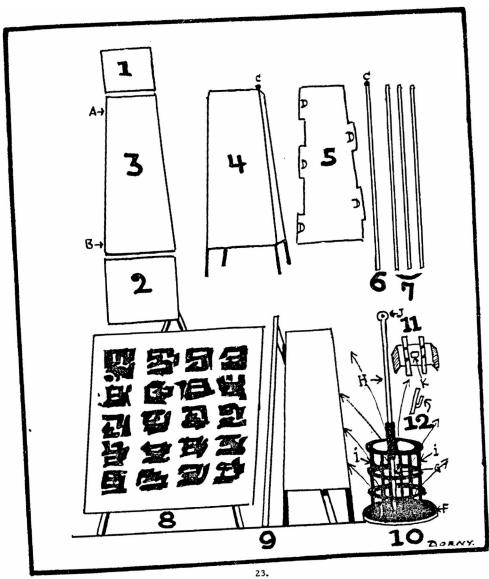
inside the cone and J is the ring in the top which passes thru K in fig. 11. The arrows show how the flower stems should be inserted in order to make them spread when the cone is removed. Fig. 11. The little sheet metal spider which fits in the top of Fig. 4. The flowers are suspended by the ring J passing thru the slot K and held in place by the pin I. The two bent ends, M,M, fit into the slots shown in figure 12.
