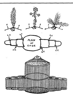
I regret that I have not drawn the plan of the cage quite accurate, for the three small cage parts should be shown broader, to allow each part to swing into each other. The arrows point to where the spring hinges are fitted.
