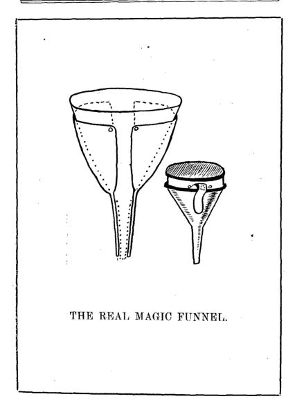
this odd space goes to make up the third division of the funnel. The third division is controlled by the hole under the top of the handle as in the ordinary funnel.
