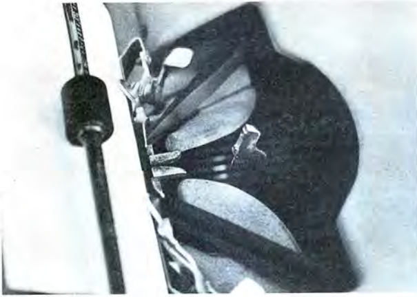
Front-striking printer: the character or dot to be printed is impressed first on the ribbon, then on the paper.
