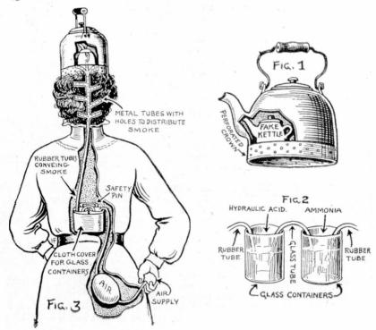
Apparatus for Smoke effect consists as follows:
