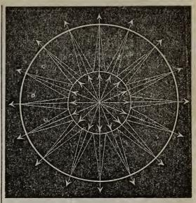
or a negative internal and a positive external surface; but if we now place the plate on the negative pole of the same battery, the order of the magnetism of the plate will be reversed as represented in this figure.
