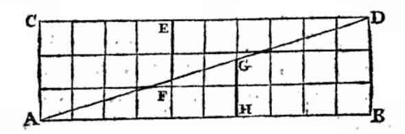
Divide the longest side into ten equal parts, and the shortest into three equal parts, and draw the perpendicular lines, as in the sigure, which will divide it into thirty equal squares.
